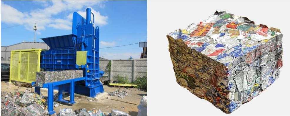
Image 7: Baling press from ATM Recyclingsystems and result can baling
