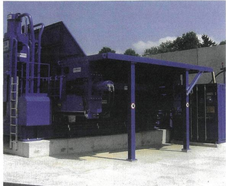
Scrap shear with baling and breaking function (Photo: ATM)
